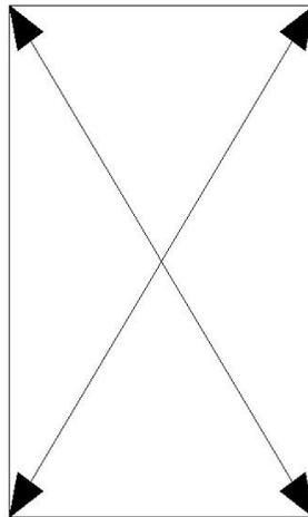
2. Using a tape measure, check the rough opening. Measure diagonally across the opening. Diagonal measurements need be equal within 1/4".
