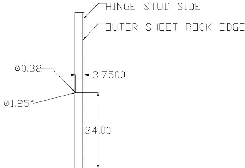
3. Referencing drawing above, drill a 3/8" thru hole in the proper location (3.75 from outer edge of sheet rock)
