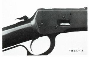
The hammer can be placed in this position in either of two ways. First, every time the lever is cycled the rearward movement of the bolt will leave the hammer in this position. The hammer may also be manually placed at full cock by pressing it rearward with the thumb until it engages the full cock notch. Be
