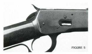
Like its nineteenth century counterpart, your Browning 92 has a full length firing pin. This means that with a cartridge in the chamber and the hammer in the dropped or fired position, one end of the firing pin will be touching the hammer and the other end of the firing pin will be resting against the primer of the cartridge. In this configuration, a sudden jar to either the hammer or the rifle could cause discharge.
