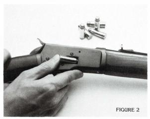
4. WITH A ROUND IN THE CHAMBER, YOU NEED ONLY THUMB THE HAMMER BACK TO ITS FULL COCK POSITION TO READY THE RIFLE FOR FIRING. Otherwise, cycling the lever to place a round in the chamber will leave the hammer in the full cock position.
