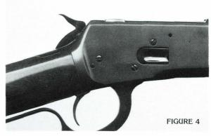
In order to move the hammer from full cock to the half cock position, you must first place your thumb on the hammer to restrict its forward movement. The trigger is then depressed to release the hammer from the full
