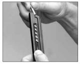
Depress the magazine's follower button with the thumb of one hand while inserting cartridges with the other hand.
