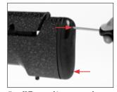
Use a Phillips screwdriver to remove the recoil pad.
