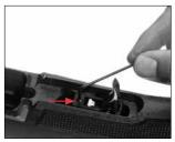
Adjust the trigger pull using a 2mm Allen wrench.
