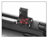
Tighten the screws incrementally in the pattern shown above.
