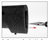
Use pliers to remove the comb retaining clip from the rear shaft of the comb.
