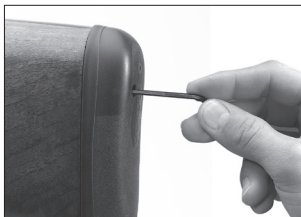
Insert a \frac{7}{64} " Allen wrench through the hole in the recoil pad.
