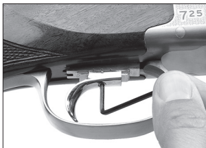
Loosen the center screw on the trigger shoe with the Allen wrench.
