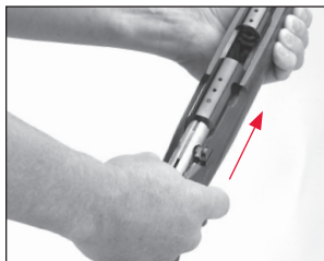
Insert the bolt into the receiver until it latches into place.
