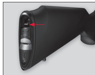
Press the magazine latch above the magazine to eject the magazine from the buttstock.
