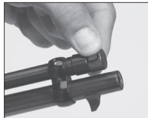
**Depress the latch and pull the magazine tube out.**
