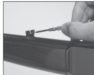
Use a small blade screwdriver to make vertical corrections to the rear sight.
