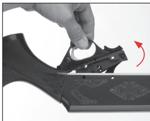
Lift the trigger group from the receiver.
