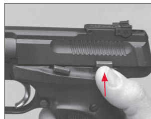
Engaging the manual thumb “safety.”
