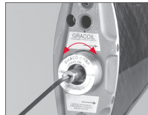
Adjust the compression unit to control the level of felt recoil.
