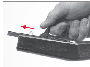
Push the trigger group forward in the receiver.
