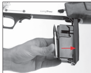
Press the cartridge into the magazine until it is retained by the magazine feed lips.
