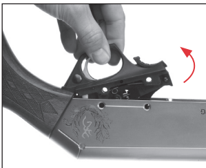
Lift the trigger group from the receiver.
